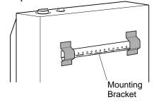
Figure 12 - Mounting Bracket Location
